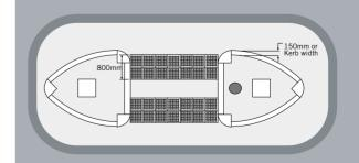
Grey or buff tactile paving should be used but with no "stems" at the following locations:
