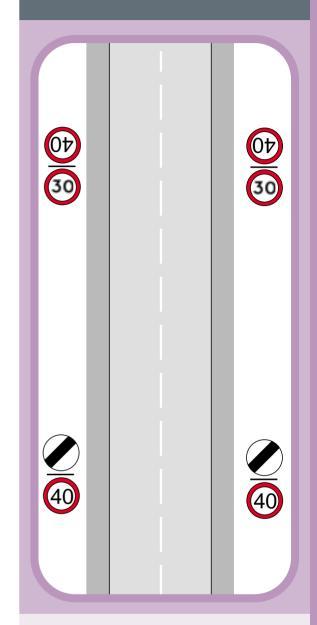
speed limit to clear a hazard such as a bend, a junction or a hump-backed bridge. The signs for the limit need to be located in a position where they can be clearly seen.
