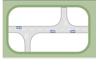
A crossroads layout can lead to a higher number of accidents than for other layouts. However it can be appropriate in low speed, low volume environments eg residential cells.
