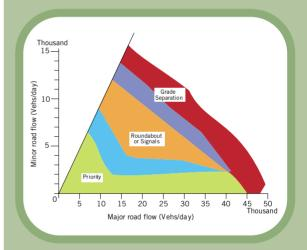
Junction choice is determined through assessment of all user needs, not just those of vehicular traffic. Traffic signals and roundabouts (including miniroundabouts) should be considered as an alternative to priority junctions when there are substantial delays to minor road traffic or where there are accident problems relating to vehicle turning movements.
