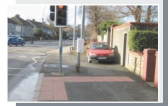
Tactile paving slabs
