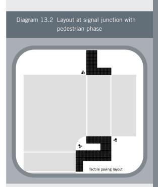
The top of the dropped kerb at the crossing should be painted white for the benefit of partially sighted pedestrians. Chamber and inspection covers should be located outside the crossing and its approaches where possible. If this is unavoidable, the tactile paving units should be laid into recessed covers to maintain the consistency of paving (see Picture 13.6). Signal controlled junctions without a pedestrian stage should be treated as uncontrolled crossings.
