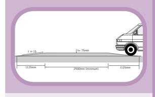
Diagram 6.35 Speed table layout at junction
