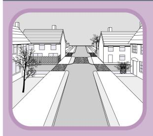
**Priority Junctions** – Drivers slow down when turning or yielding right of way at junctions. The careful positioning of priority junctions can assist in restraining speed along a length of road (see Diagram 7.8). Crossroads layouts are not recommended.
