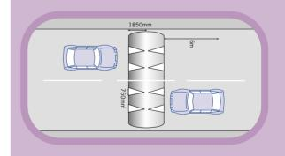
marking is commonly used across the whole width of the measure. In Ireland a variety of markings have been used in recent years. It is the responsibility of each road authority to satisfy itself that the markings used are clear and unambiguous. The signs and markings should be positioned so that parked vehicles do not obscure their visibility.
