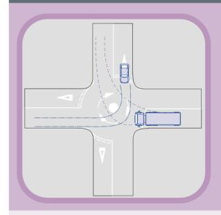
On roads where 85% speeds are between 30mph and 40mph the following features should be incorporated into the design to reduce approach speeds and alert drivers to their presence (see Diagram 6.15):
