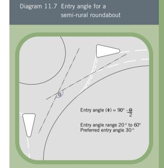
the junction and encourage high entry speeds in light traffic conditions. Where more than one lane is provided, lane widths should be between 3m and 3.5m at the entry yield line.
