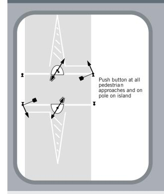
Detectors can be mounted on the traffic signal heads. These detect gaps in traffic and allow an earlier introduction of the green man crossing if there is a gap in traffic
