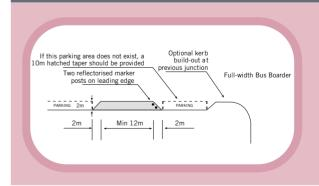
where kerbside parking space is at a premium or where it occurs with vehicles either parked at an angle or at right angles to the kerb. Bus promontories give passengers a protected route through the parked vehicles to the raised kerb. However, the disadvantage is that passenger waiting facilities cannot be provided immediately adjacent to the bus stop. They can generally be used only with single-door, front entrance buses.
