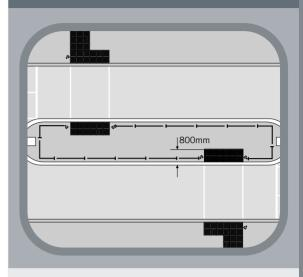
Diagram 13.7 Layout for raised entry treatment at a junction
