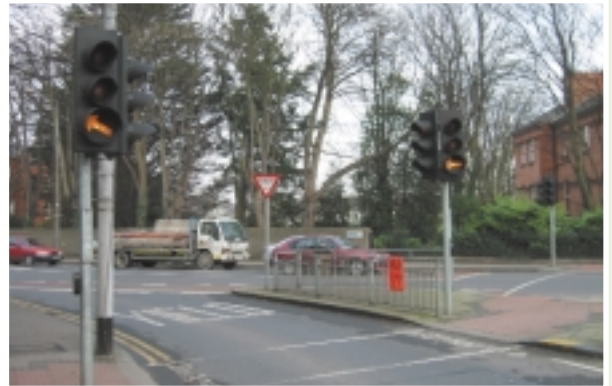
Flashing amber for turning vehicles
